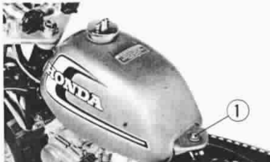
① Setting 6 mm bolt Fig. 49
